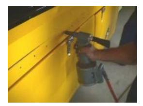
Inserting stainless steel rivets through flange to body. \*Note: Longer rivets must be used when securing the compartment door hinges to make sure that they contact the metal bodywork.
