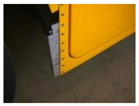
Install the rear luggage trim plate. This item is not supplied on conventional buses (customer manufacture) from 16ga satin coat steel.
