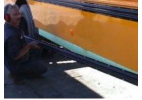
Removing the lower rub-rail. On cut-out of the box, plus 2-4" to allow for box flange as described in previous section.
