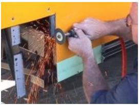
Where the substructure is overlapped a cutting tool is needed to cut through both layers. A die grinder is recommended (air or electric\*)
