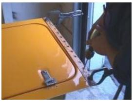
Using a template, or by measuring and marking off equally space points, the upper and two side flanges are drilled. Side holes should be 4.1/2" apart approx. Upper mounting flange should 4 7/8" Note\* To ensure spacing is equal, lay out top and sides before drilling.
