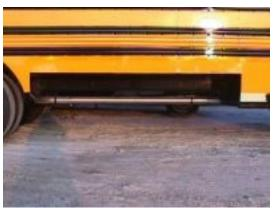
The body is now ready for the installation of the luggage compartment. At this point all unpainted edges should be treated or painted to prevent future corrosion. Marking and drilling the holes for the rear luggage support brackets. Approximately 5" from the bottom of the box.
