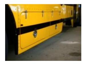
To finish the installation, a bead of yellow silicone may be applied to the outer edge of the compartment. And install black vinyl tape if required. It is recommended not to apply tape over rivets and silicone.
