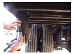
Removing the body panel support gussets. \*Note: It is acceptable to cut the gusset and not remove the rivets.
