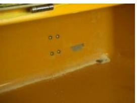
It is secured in place by four carriage bolts.
