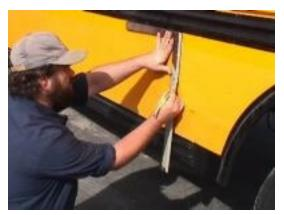
On all installations the lateral cut in the body Should be level with the lower edge of the Floor cross members. (Approx 36" from Ground level) The vertical cuts in the body should be as Wide as the luggage compartment. And the box should be located centrally without impairing any of the chassis or body components.
