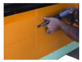
Using an air chisel to remove the rivets in body panels. \*Note: The two center rivets above the marked cut out area are removed to allow room for the luggage compartment outer flange.
