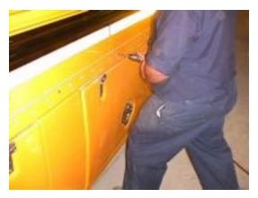
The body is drilled using the holes in the flange as a pattern.
