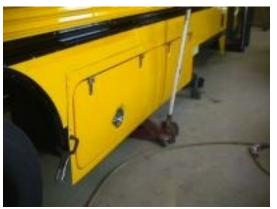
The compartment is positioned in the cut-out supported by a jack, when the compartment is in the correct position it is clamped at the sides.
