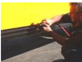
Using a high speed cutting disc, cut the rub rails. Safety Glasses should be worn. As described below.
