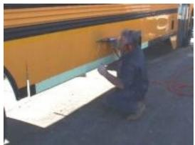
With all the rivets removed, a centre drop tooth PH51D (Snapon) tool is used in the air gun to remove the upper panel only\*,
