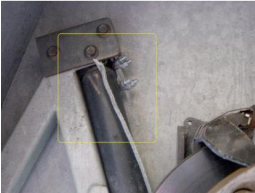
BROKEN SUSPENSION TRAVEL LIMIT CABLE (422 TEST MILES)
