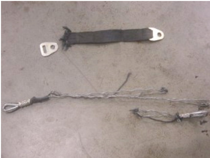
BROKEN SUSPENSION TRAVEL LIMIT CABLE (3,831 TEST MILES)
