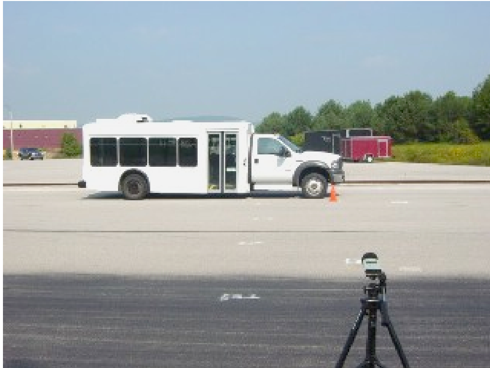
TEST BUS UNDERGOING EXTERIOR NOISE TESTING
